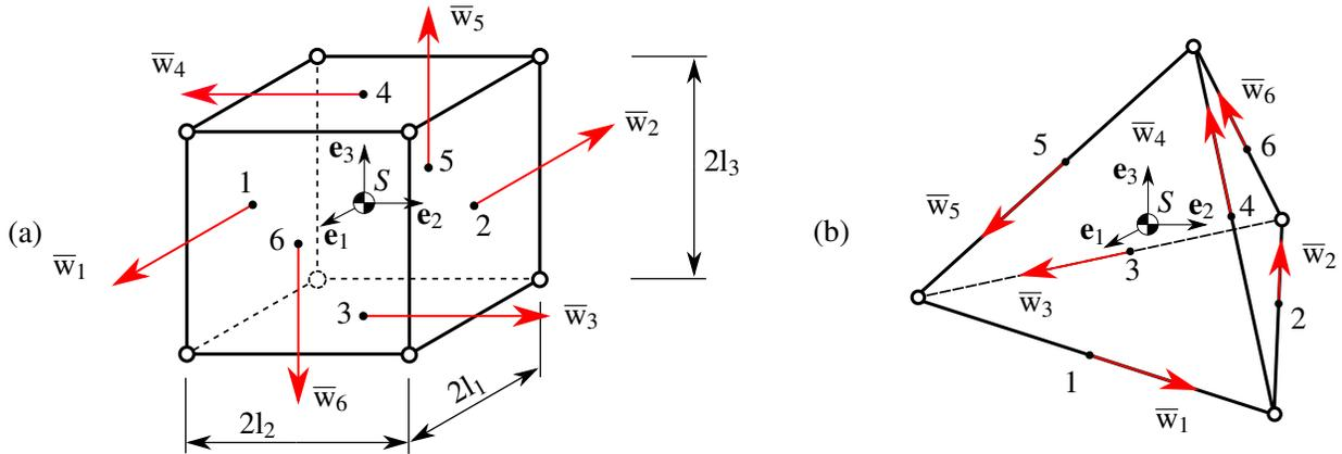
Fig. 4: Basic geometries for unified local velocity coordinates.  $S$  denotes the center of mass of the rigid body. The six points, used for the velocity projection are denoted with  $1 \dots 6$ . The corresponding six unified velocities are denoted by  $\bar{w}_1 \dots \bar{w}_6$ . Fig. a) shows the hexahedral case, Fig b) shows the tetrahedral case.
