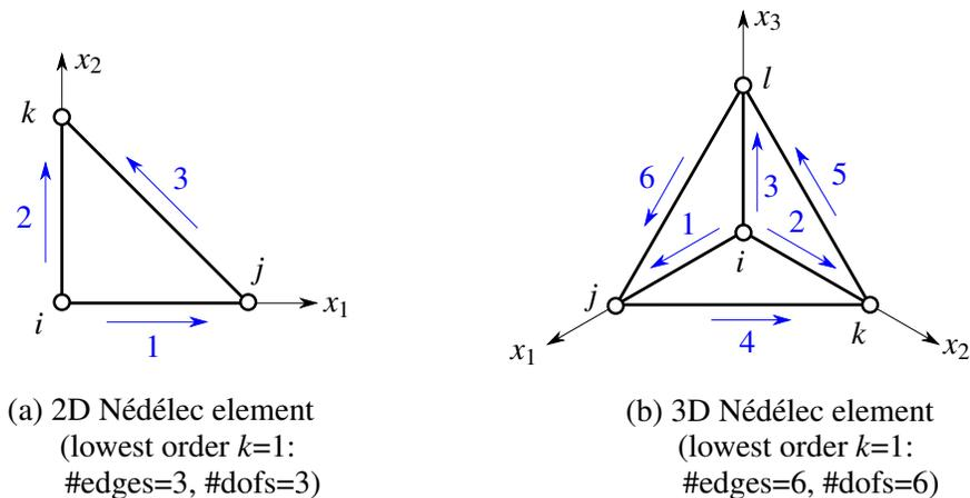
Fig. 1: Degrees of freedom of a Nédélec element of 1st-kind.
