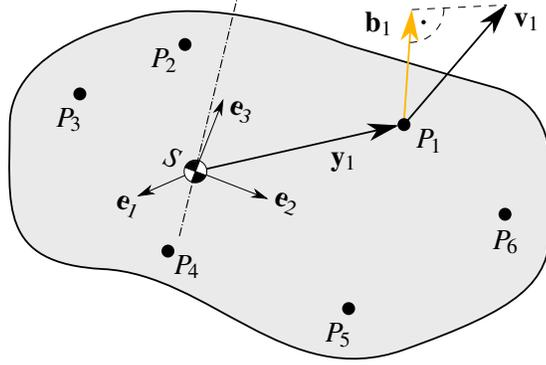
Fig. 3: Basic projection idea to obtain unified local velocity coordinates.  $S$  denotes the center of mass of the rigid body. The six points, used for the velocity projection are denoted with  $p_1 \dots p_6$ . Note that  $\mathbf{b}_1, \mathbf{v}_1, \mathbf{y}_1$  and  $\mathbf{e}_i$  are the global representations of their body-fixed counterparts  $\tilde{\mathbf{b}}_1, \tilde{\mathbf{v}}_1, \tilde{\mathbf{y}}_1$  and  $\tilde{\mathbf{e}}_i$ .
