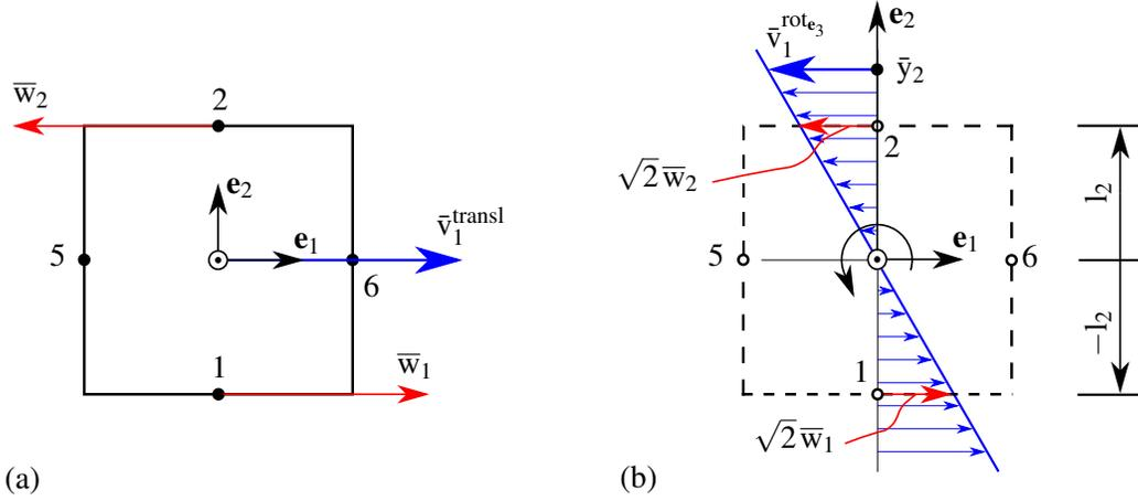
Fig. 5: Representation of the motion of the cross-section spanned by the transformation points (1,2,5,6), see also Fig. 4 a.
