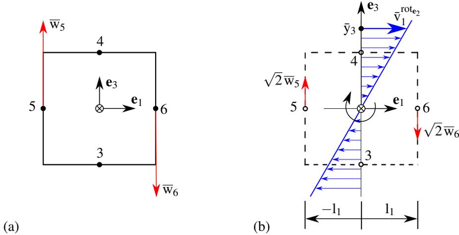
Fig. 6: Representation of the motion of the cross-section spanned by the transformation points (3,4,5,6), see also Fig. 4 a.
