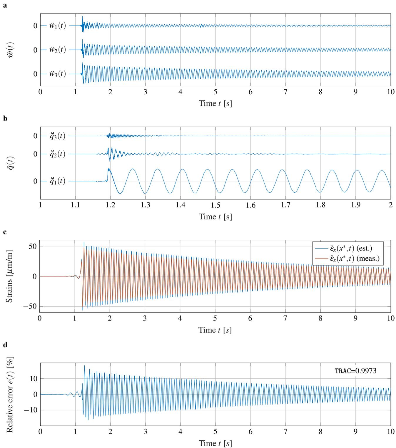
Fig. 5: Results of free vibrations test. **a** Normalised acceleration measurements  $\ddot{w}(t)$  at locations  $x_k$ ,  $k = 1, 2, 3$  **b** Normalised decomposed modal accelerations  $\ddot{q}(t)$  **c** Estimated and measured strains at location  $x^*$  **d** Relative error  $e(t)$
