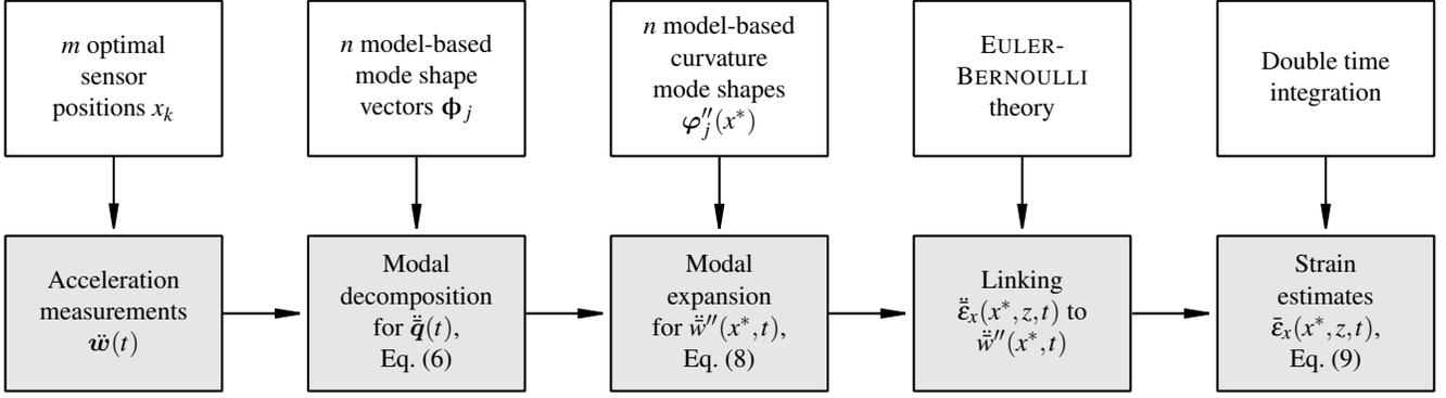
Fig. 2: Required steps for strain estimations on the basis of MDE
