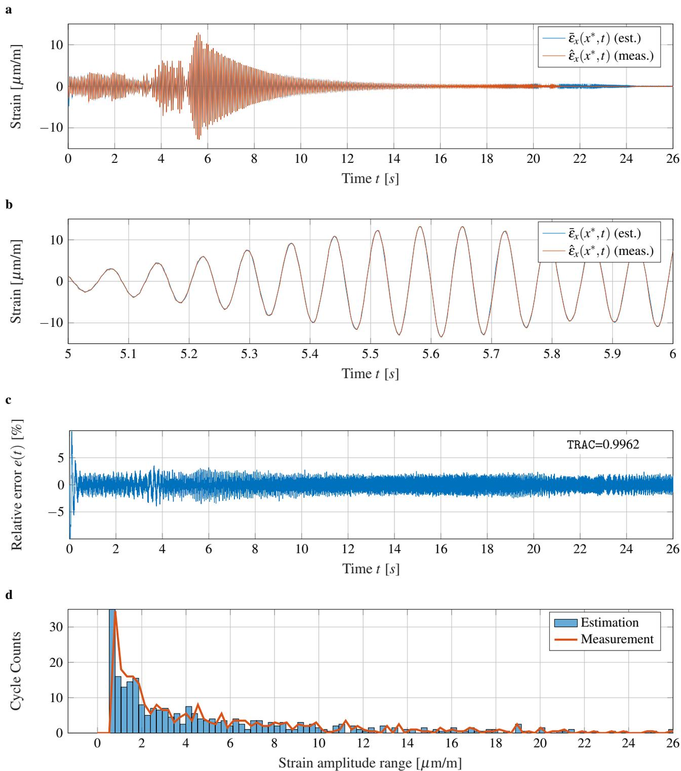
Fig. 8: Results of forced vibrations test under sweep excitation; MDE on basis of beam model with clamping stiffness. **a** Estimated and measured strains at  $x^*$  **b** Enlarged section of strain time history **c** Relative error  $e(t)$  **d** Rainflow histogram of strain time histories
