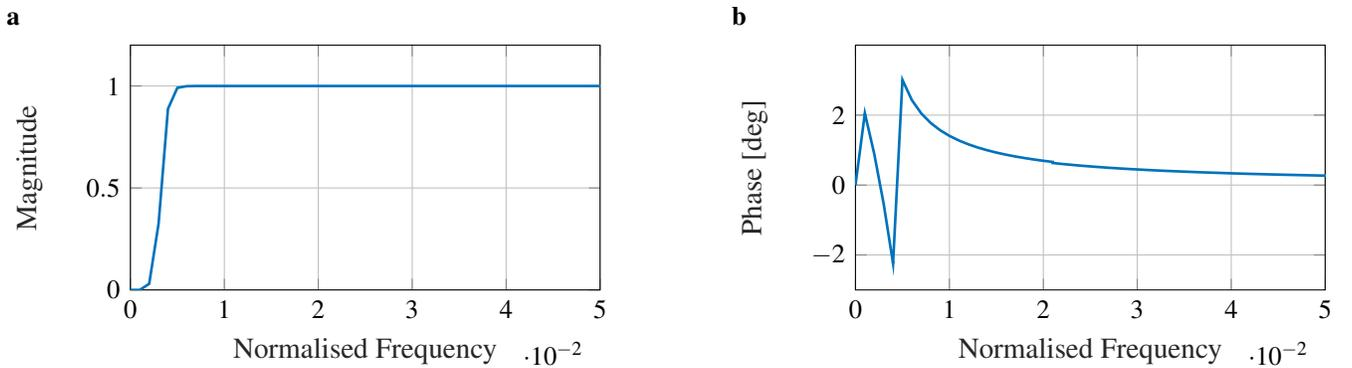
Fig. 3: Frequency response of 6<sup>th</sup> order Butterworth high-pass filter with  $f_{\text{cut}} = 7\text{Hz}$ ; frequency normalised by Nyquist rate  $f_N = 2560\text{Hz}$ . **a** Magnitude plot. **b** Phase plot.
