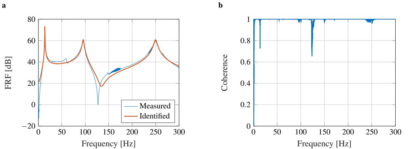
Fig. 6: Selected results of Experimental Modal Analysis. **a** One specific measured FRF and the identified frequency response. **b** Corresponding coherence.
