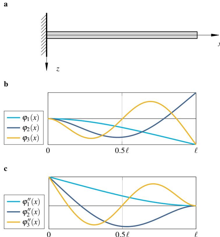
Fig. 1: **a** Cantilever beam model of length  $\ell$  **b** The first  $n = 3$  uni-axial bending mode shapes **c** The corresponding strain mode shapes.
