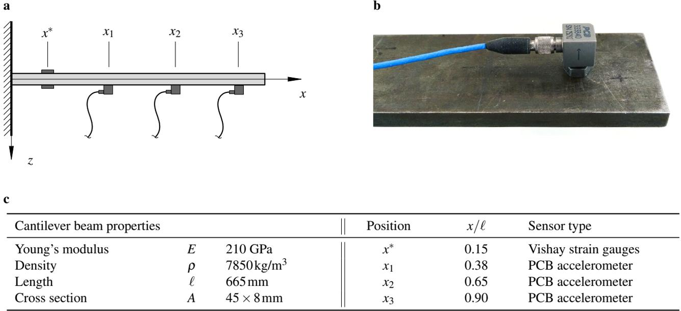
Fig. 4: Experimental setup. **a** Sensor locations on the cantilever beam with accelerometers at positions  $x_k$ ,  $k = 1, 2, 3$  and strain gauges at position  $x^*$ . **b** PCB accelerometer mounted on the beam structure. **c** Experimental setup parameters.
