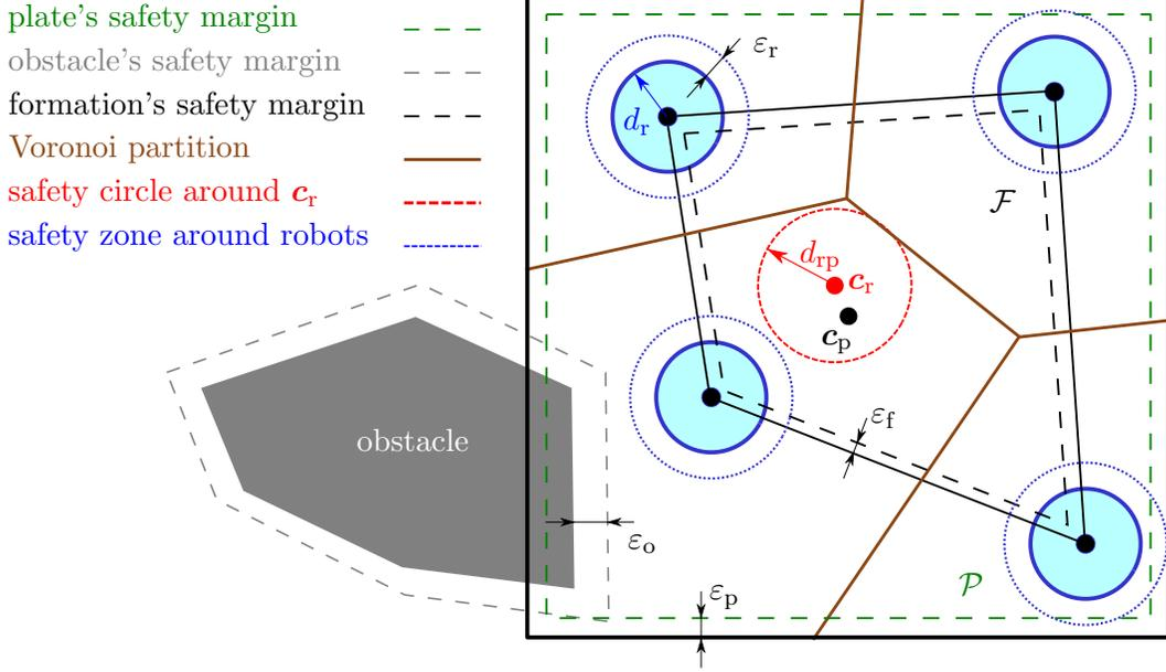
Fig. 3: Schematic of transporting a plate with conditions.
