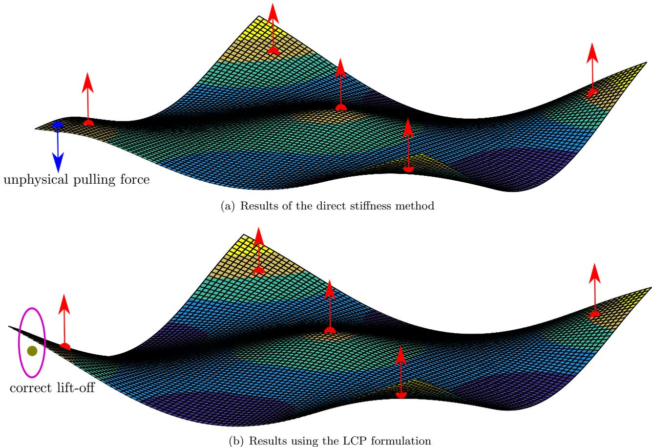
Fig. 2: Calculation of the normal forces by LCP and the direct stiffness method, from [8].
