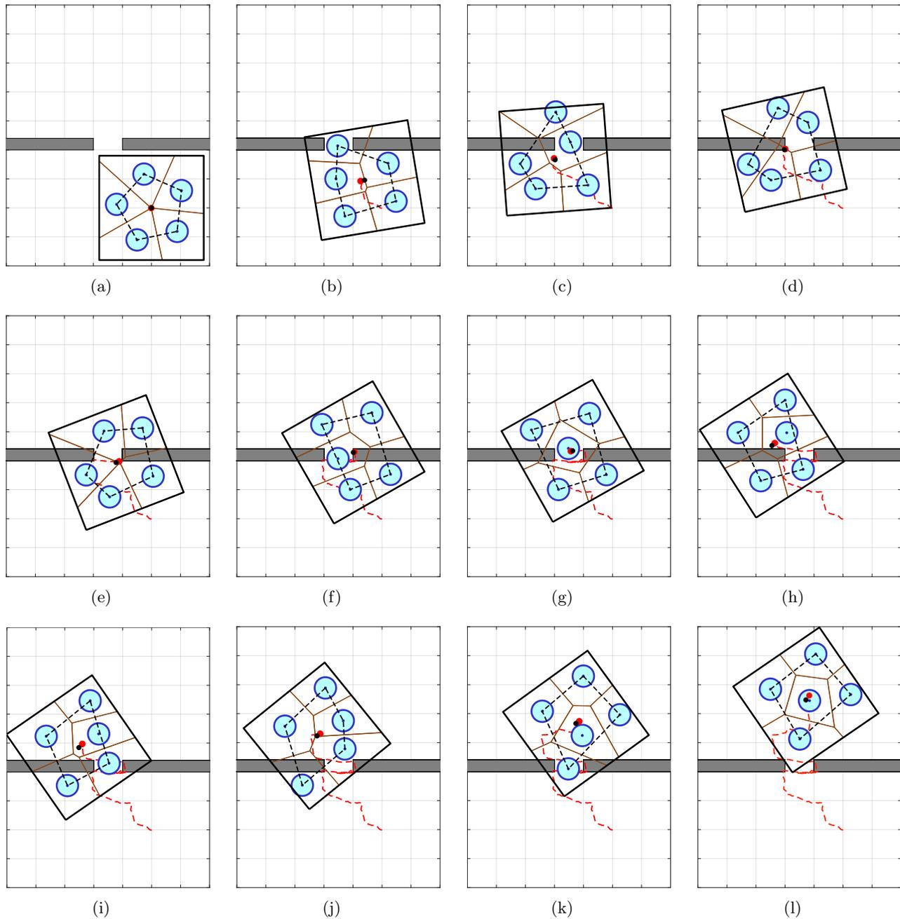
Fig. 5: Transporting an elastic plate through a narrow passage.
