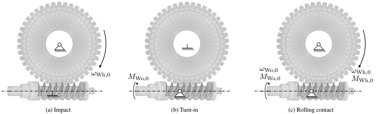
Fig. 7: Initial setup of the simulation examples
