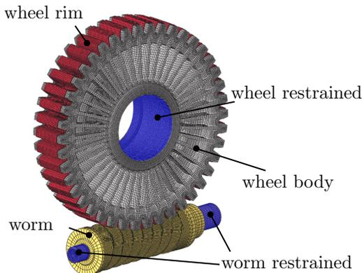
Fig. 6: Parts of the worm gear model
