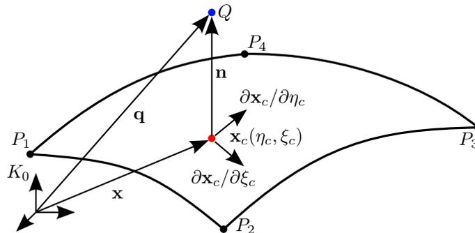
Fig. 5: Evaluation of a quadrilateral master-slave contact element
