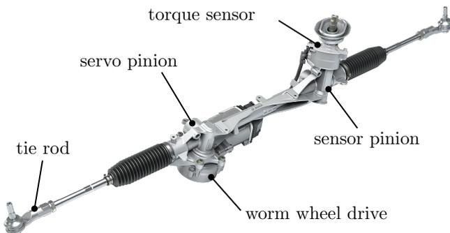
Fig. 1: EPSdp system with servo pinion [1]
