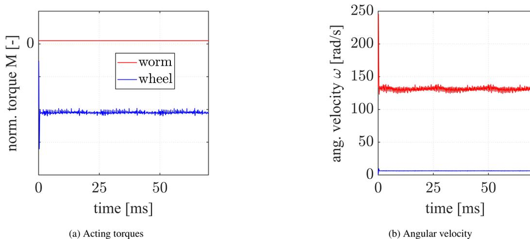
Fig. 14: Rolling contact simulation for embs1000
