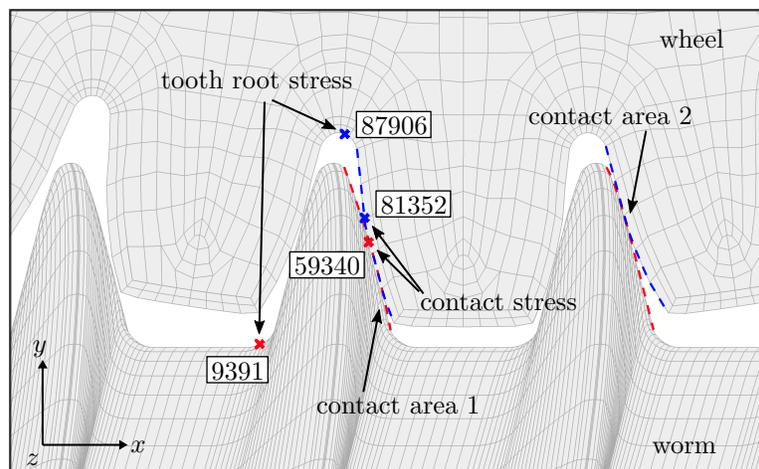
Fig. 8: Spots of stress evaluation at tooth roots and on tooth flanks
