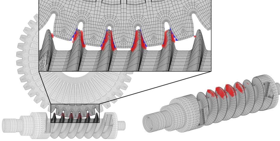
Fig. 4: Resulting k-DOPs of a binary tree search on the worm gear model; red: resulting k-DOPs of the worm, blue: resulting k-DOPs of the wheel
