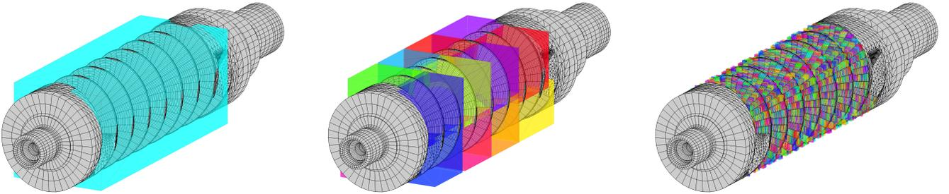
Fig. 3: Different BVH tree levels of an enveloped worm geometry; left: level 1, middle: level 5, right: level: 14/15 (leaf level)
