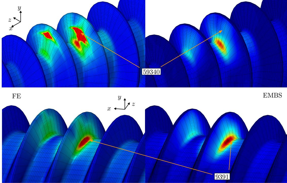
Fig. 13: Comparison of qualitative von Mises stress distribution between FE (left) and EMBS (right) on the worm gear at equilibrium
