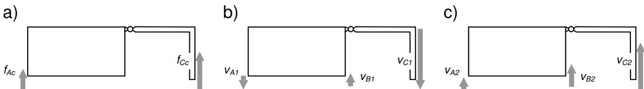
Fig. 2: Considered system: sketch of its physical model (a); initial contact velocities and the resulting contact forces (b)
