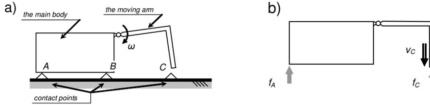
Fig. 1: Considered system: sketch of its physical model (a); initial contact velocities and the resulting contact forces (b)
