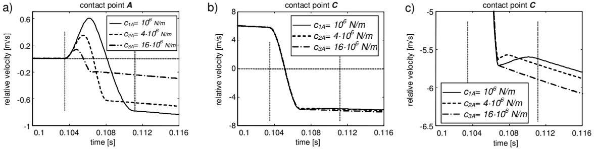
Fig. 9: Velocities of the relative penetration between the colliding bodies and the ground: contact point A (a); contact point C (b); contact point C (zoom) (c)
