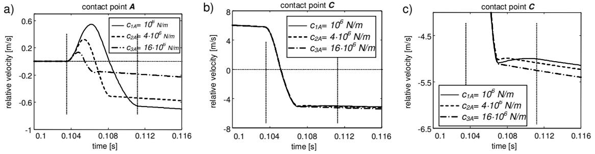
Fig. 11: Velocities of the relative penetration between the colliding bodies and the ground: contact point A (a); contact point C (b);
