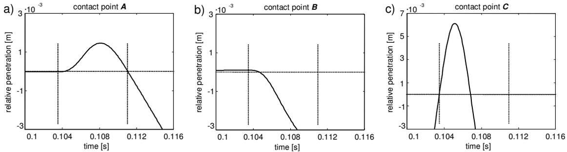
Fig. 6: Relative penetration between the colliding bodies and the ground: contact point **A** (a); contact point **B** (b); contact point **C** (c)
