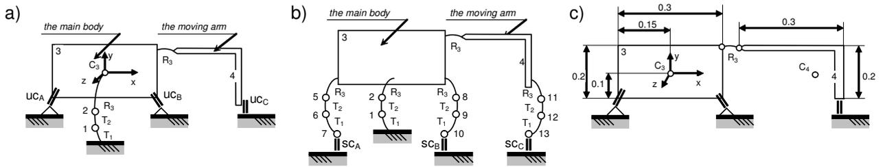
Fig. 5: Multibody structure of the considered system: reference structure (a); the modified structure devoted to model the smoothed contacts (b); the main geometrical parameters (c)
