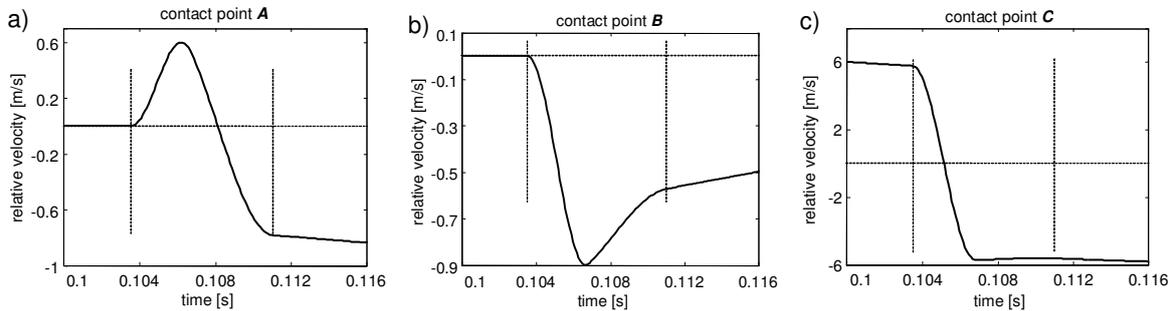
Fig. 7: Velocities of the relative penetration between the colliding bodies and the ground: contact point **A** (a); contact point **B** (b); contact point **C** (c)
