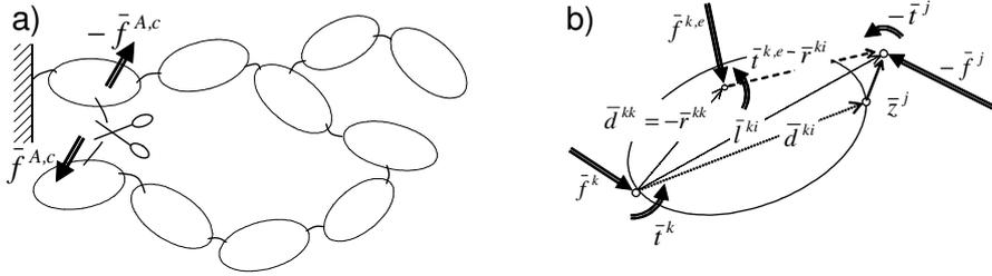
Fig. 4: Cutting procedures: reference tree structure and the cutting place (a); geometrical dimensions present at body  $\#k$  and interactions acting on the cut out body  $\#k$  (b);
