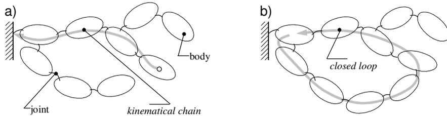
Fig. 3: Considered example multibody system: elements of the considered tree-like multibody system (a); closed loop multibody system (b);
