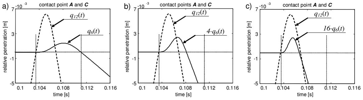
Fig. 8: Relative penetration between the colliding bodies and the ground:  $c_{1A} = 10^6 \text{ N/m}$  (a);  $c_{2A} = 4 \cdot 10^6 \text{ N/m}$ ;  $c_{3A} = 16 \cdot 10^6 \text{ N/m}$  (c)
