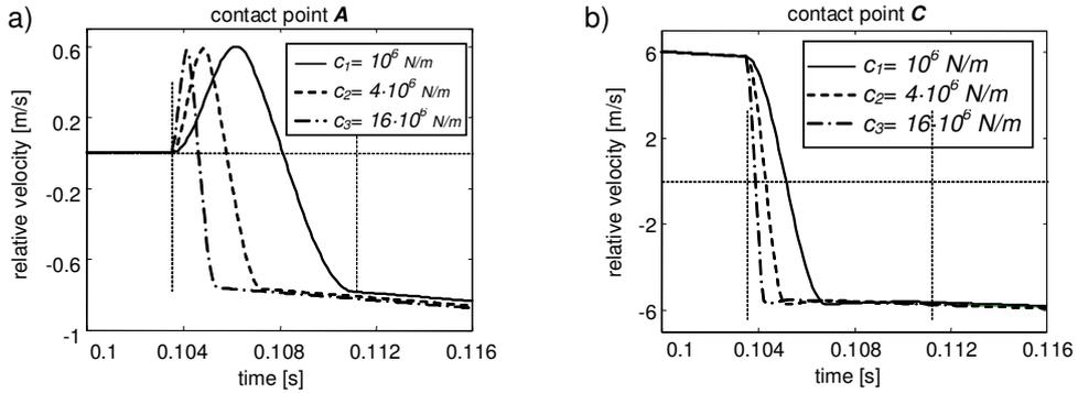
Fig. 10: Velocities of the relative penetration between the colliding bodies and the ground: contact point A (a); contact point C (b);
