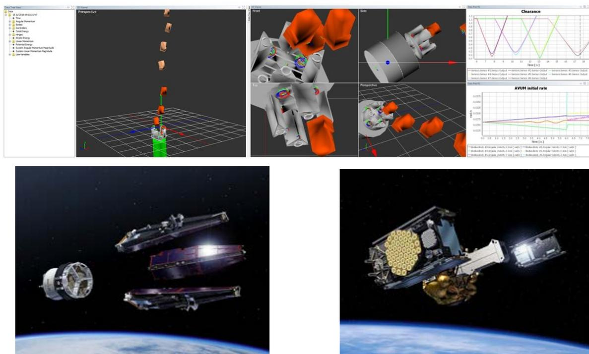
Fig. 2: Multi-payload separation study case (Credits: ESA/CNES/ARIANESPACE)
