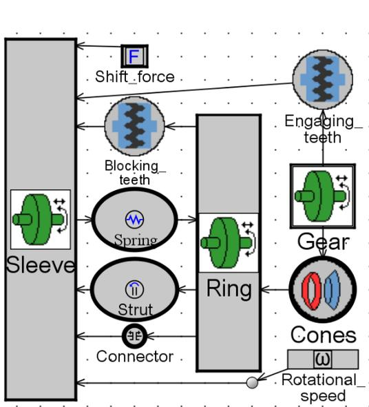
Figure 1: Gear shifting mechanism in GT-Suite.
