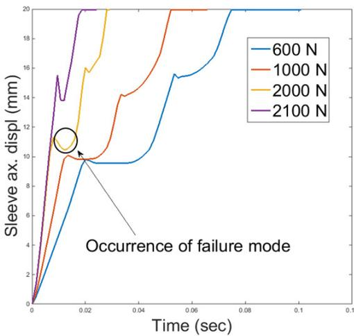
Figure 2: Sleeve axial displacement with varying shift force.
