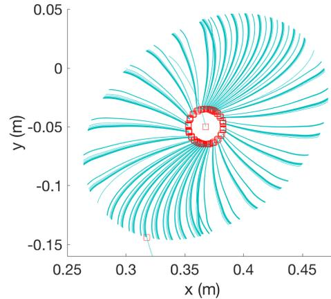
(b) The trajectories of center of mass of the pushed object in simulation result.
