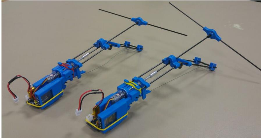
Fig. 2: Jumping robots modified with propeller looking extension allowing them to turn
