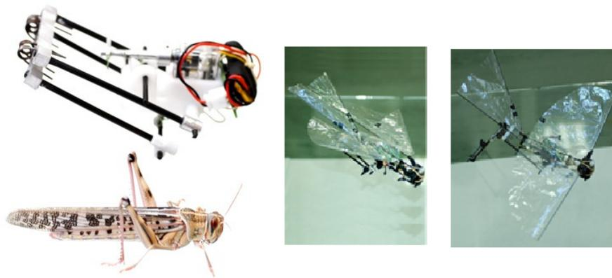
Fig. 1: Left: Locust inspired robot above a real locust. Right: Winged version
