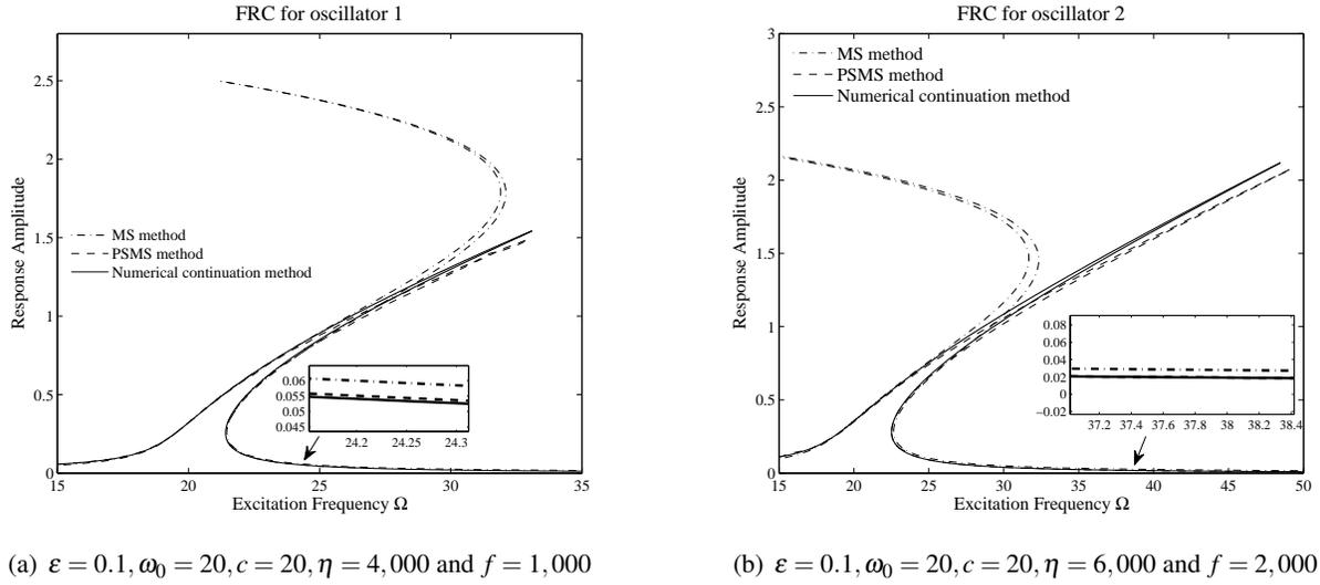
Fig. 1: The FRCs obtained by the MS method, the PSMS method and the numerical continuation method.
