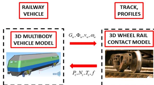
Fig.1: Architecture of the multibody model
