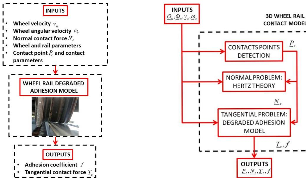
Fig.2: Inputs and outputs of the degraded adhesion model and architecture of the wheel-rail contact model
