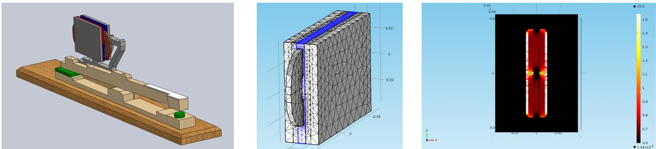
Fig. 2: Design of one-key active feedback device : 3D current CAD view (left) - FEM mesh in COMSOL<sup>®</sup> of the voice coil actuator (middle) - Magnetic field in the system (right)
