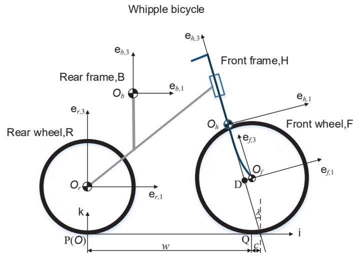
Fig. 1: The benchmark Whipple bicycle in an upright, straight reference configuration (a figure adapted from [4]).
