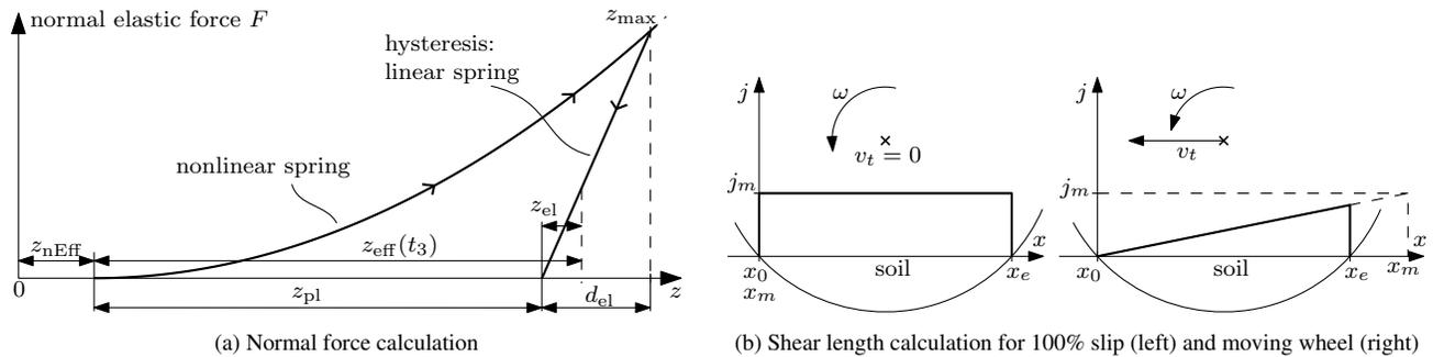
Fig. 1: Schematics of normal force and shear length in TerRA
