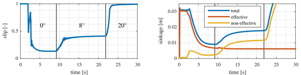
Fig. 2: Wheel slip (left) and sinkages (right) for verification scenario
