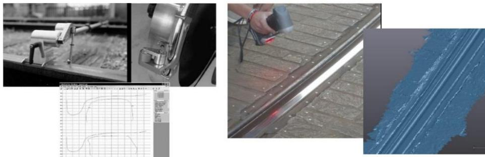
Fig. 1 Example of 2D and 3D measuring instruments and profiles acquired
