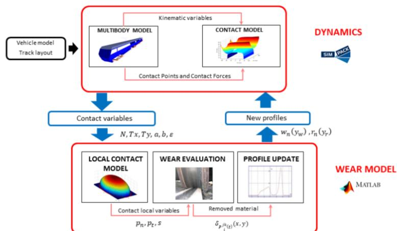
Fig. 2 Wear model general layout
