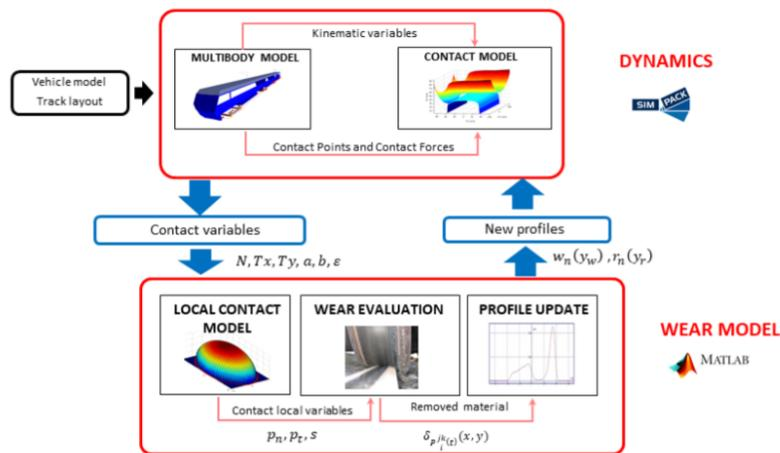
Fig. 2 Wear model general layout
