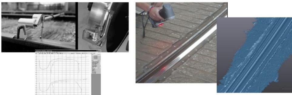
Fig. 1 Example of 2D and 3D measuring instruments and profiles acquired
