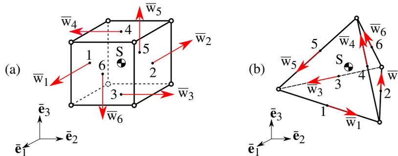
Fig. 1: Basic geometries for unified local velocity coordinates. S denotes the center of mass of the rigid body. The six points, used for the velocity projection are denoted with 1...6. The corresponding six unified velocities are denoted by  $\bar{w}_1 \dots \bar{w}_6$ . Fig. a) shows the hexahedral case, Fig b) shows the tetrahedral case.
