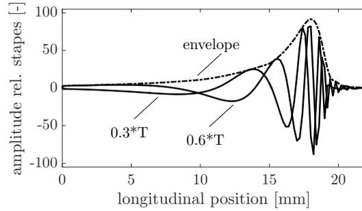
Fig. 1: Transversal amplitude of the basilar membrane relative to that of the stapes footplate for two different points of time of a cycle for an excitation frequency of 1 kHz
