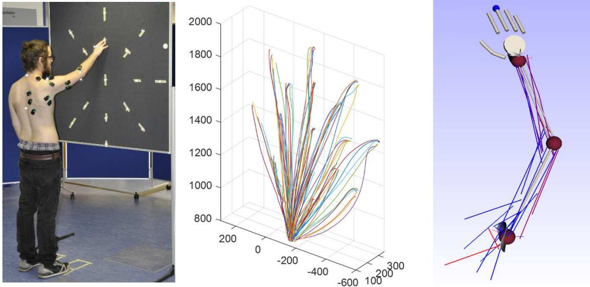
Fig. 1 *left*: the basic reaching test in the motion lab *middle*: measured hand trajectories for certain target points; *right*: simulation of a reaching task with our DHM arm Model (upper arm, forearm and hand modeled as rigid bodies (grey) connected via joints (5 DOF, red balls with grey ellipsoids delimiting the range of motion) and actuated by hill-type muscle models (blue and red lines, 29 muscles)
