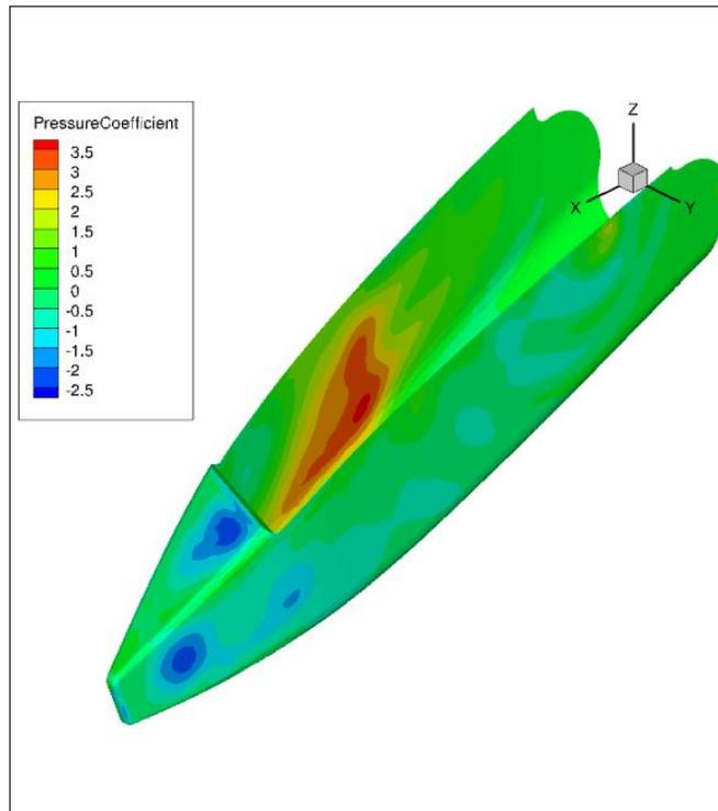
Fig. 3: Pressure coefficient on the outboard fairing surface only at time  $t = 0.042s$ .
