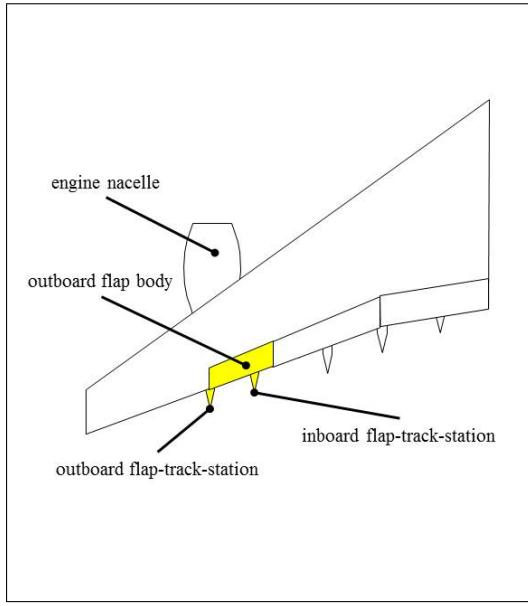
Fig. 1: High-lift system of a commercial aircraft.
