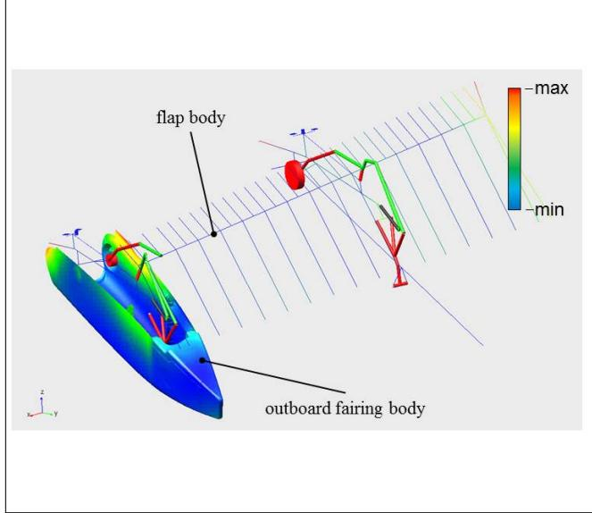
Fig. 2: Deformations of the outboard fairing body from Adams simulations: outboard view. Deformations are normalized respect to the highest deformation value. Ascending level of deformation intensity from blue (min) to red (max).
