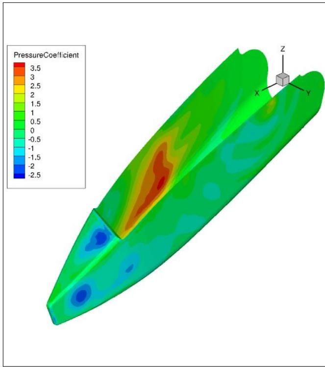
Fig. 3: Pressure coefficient on the outboard fairing surface only at time  $t = 0.042\text{s}$ .
