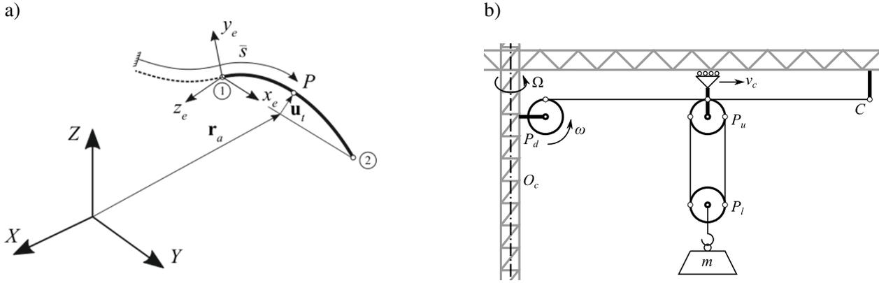
Fig. 1: a) Body frame and arbitrary displacement vectors in an ALEM segment. b) Simplified crane model.
