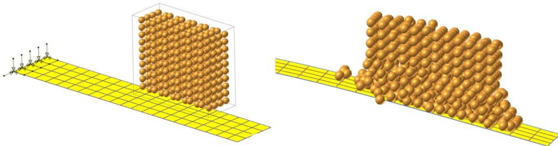
Fig. 2: Coupled simulation with flexible shell specimen and particles
