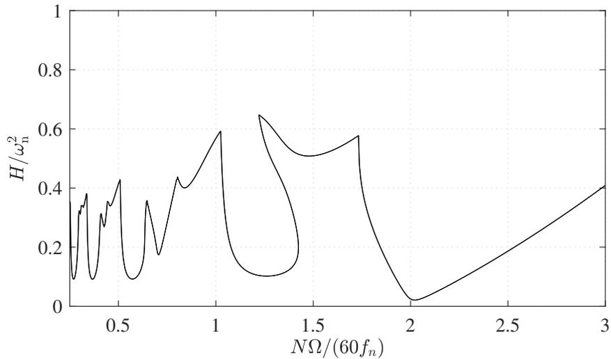
Fig. 1: Stability lobe diagram of full-immersion milling with a single-degree-of-freedom model in the space of the technological parameters spindle speed  $\Omega$  and specific cutting-force coefficient  $H$ , for details see [7]
