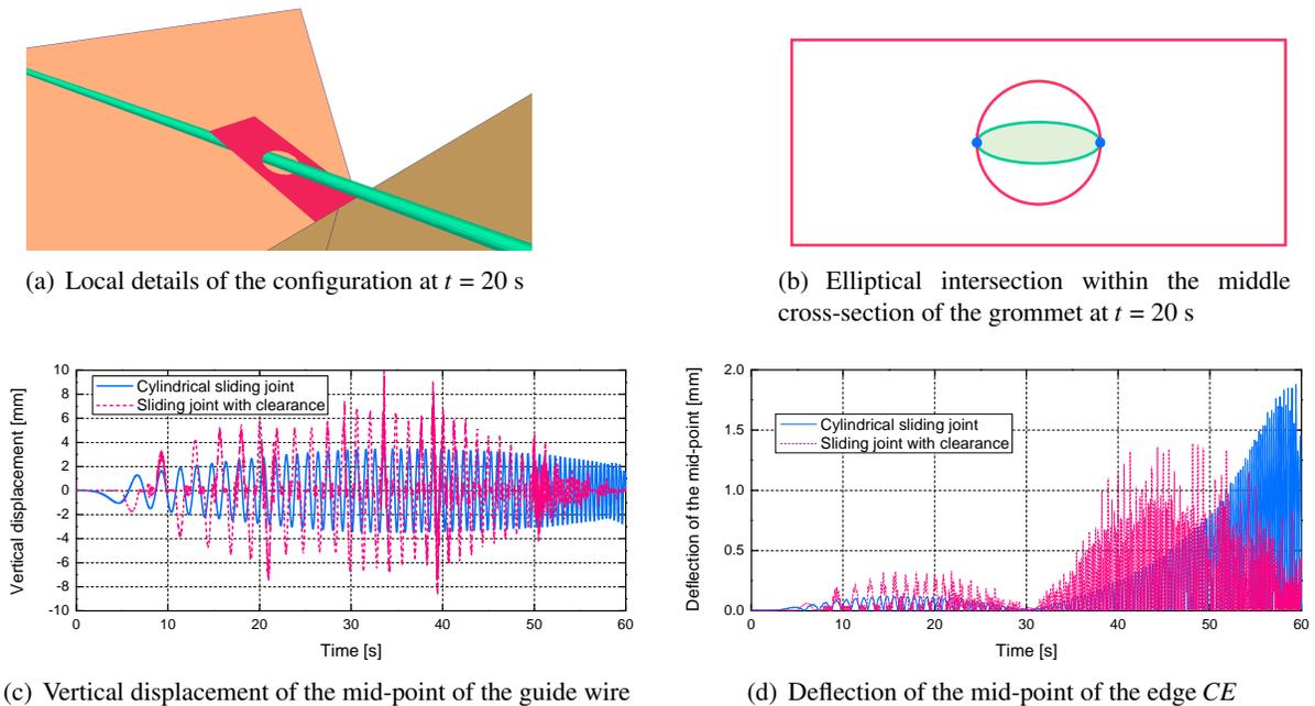
Fig. 2: Dynamic responses of the simplified model of the solar array wing
