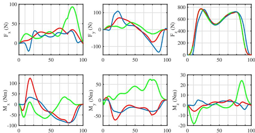
Fig. 1: Ground reaction forces and moments in global coordinates. X: lateral-medial direction. Y: anterior-posterior direction. Z: vertical direction. Moments referred to the center of the force plates. In blue, provided by the force plates. In red, obtained as the solution of the inverse dynamic problem using UNO. In green, obtained as the solution of the inverse dynamic problem using GOM
