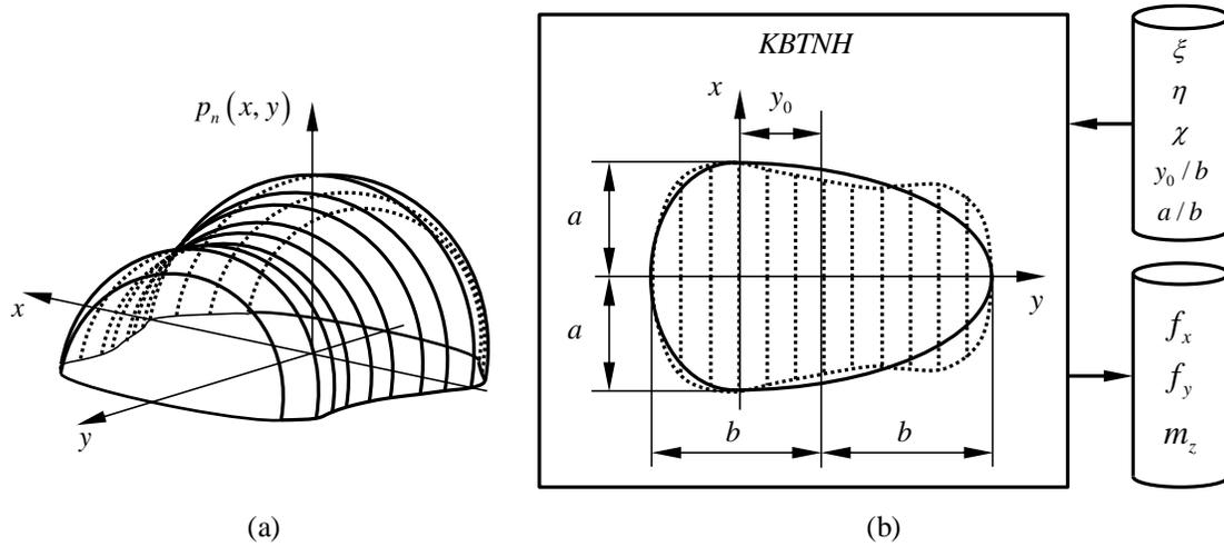
Fig. 2: (a) Normal pressure distribution for an arbitrary contact patch [5] and (b) creepage forces obtained from the Kalker Book of Tables for Non-Hertzian (KBTNH) contact patches [6]
