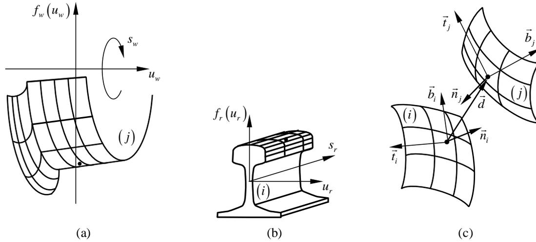
Fig. 1: Parameterization of the (a) wheel and (b) rail and (c) contact detection between surfaces
