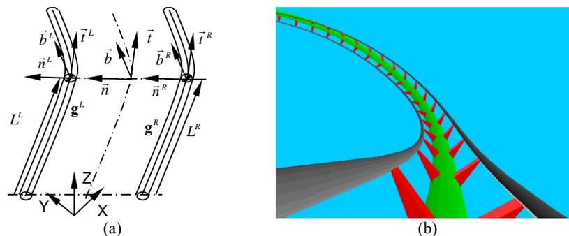
Fig. 1: Spatial description of the roller coaster rails: (a) Frenet and rails moving frames: (b) Geometry of the rails for a roller coaster.
