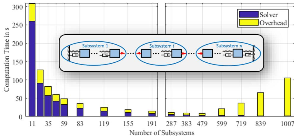
Fig. 1: Computation time of a co-simulation using a various number of subsystems (overall system: multibody system with 1.0e6 degrees of freedom)
