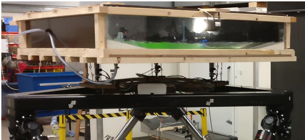
Fig. 1: Experimental TLD mounted on a MOOG MB-E-6DOF/24/1800kg motion base.
