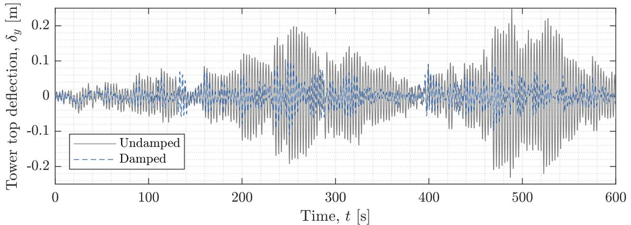
Fig. 2: Damping of lateral tower top deflections at a mean wind speed of  $15 \text{ m/s}$  at hub height.
