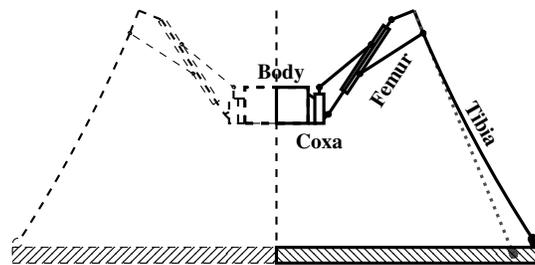
Fig. 1: Schematic diagram of the leg system of MAX
