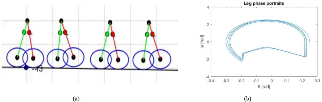
Fig. 1: (a) Passive biped-walking robot multibody model; (b) Leg phase portraits
