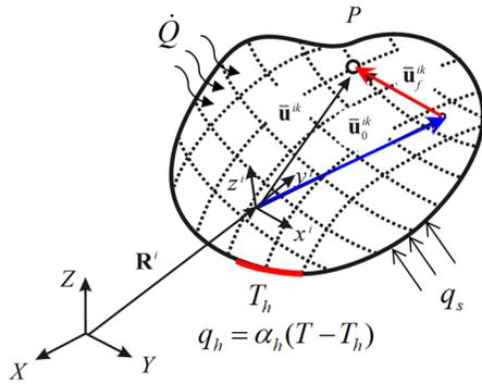
Fig. 1: Thermomechanical coupling model using the floating frame of reference formulation
