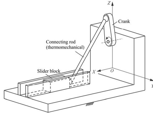
Fig. 2: Spatial slider crank mechanism with thermomechanical connecting rod model
