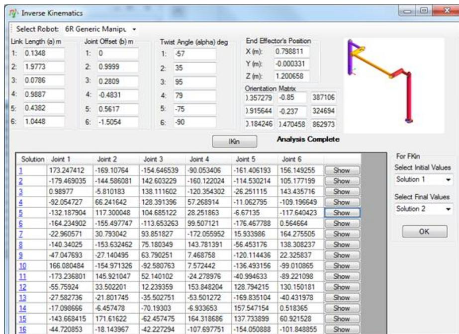
Fig. 1: Inverse Kinematics module in RoboAnalyzer for general 6R manipulator
