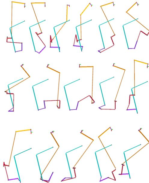
Fig. 2: 3D representation of the 16 distinct inverse kinematic solutions
