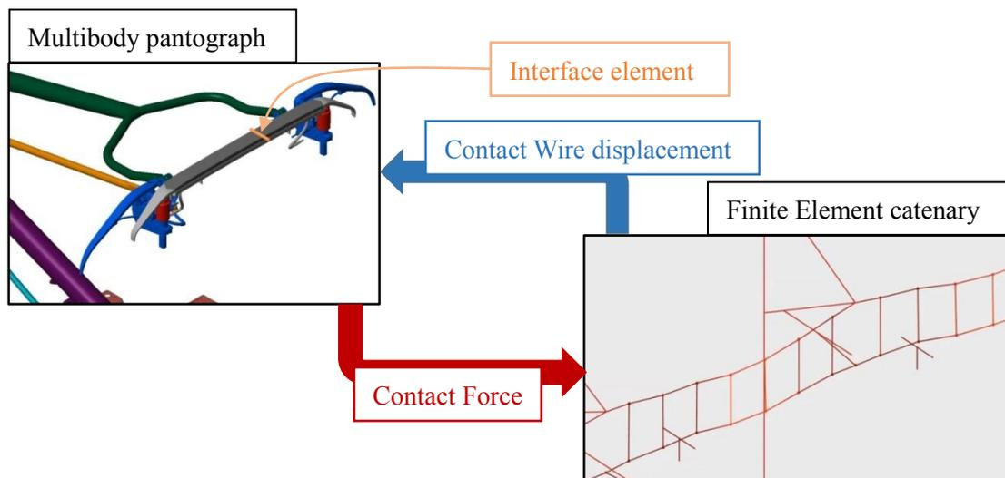
Fig. 1: The FE solver transfers contact wire displacements to an interface element in the MBD software. In return the contact force between the interface element and the pantograph contact strip is sent back to the FE solver to compute the next time step.
