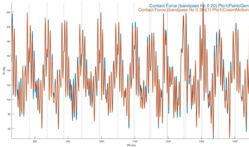
Fig. 2: Comparison of co-simulation results for a given pantograph catenary configuration (two pantographs raised on the same train 200 m apart at 300 km.h<sup>-1</sup> on a high speed 25 kV line). Evolution of contact force with train position. The red curve shows the co-simulation results and the blue curve shows the FE only results both filtered at 20 Hz.
