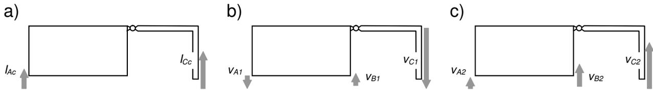
Fig. 2: Impacts and velocities at the impacting points: detected impacts (a) velocities at the initial period of compression (b) velocities at the final period of expansion (c)
