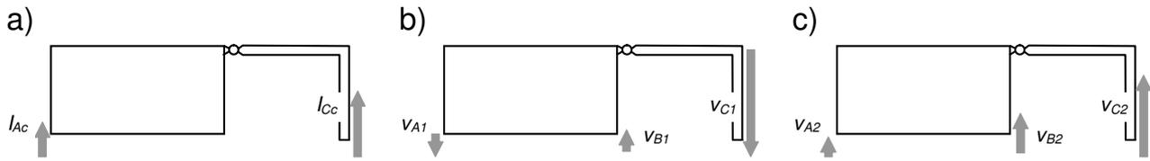
Fig. 2: Impacts and velocities at the impacting points: detected impacts (a) velocities at the initial period of compression (b) velocities at the final period of expansion (c)
