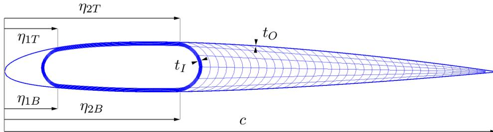
Fig. 1: Example shape parameters in blade cross-section
