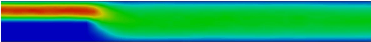
Fig. 3: Backward facing step results for the SPH projection method without the consistent formulation of Eq.5.
