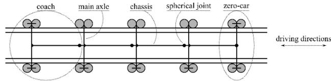
Fig. 1: Schematic top view of a roller coaster train with four coaches, connected to a zero-car
