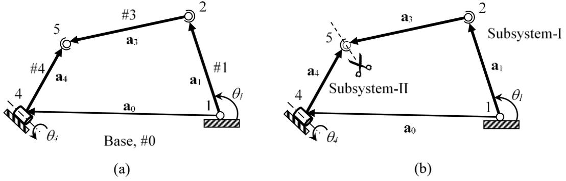
Fig. 1: RSSR mechanism
