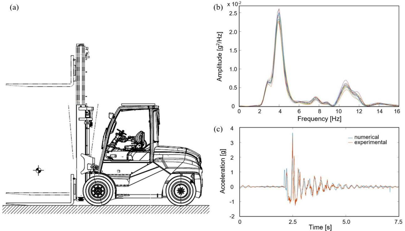
Fig. 1: (a) Schematics of the forklift, (b) power spectra of the acceleration signals of the left front wheel hub, (c) comparison between experimental measurements and updated numerical model.
