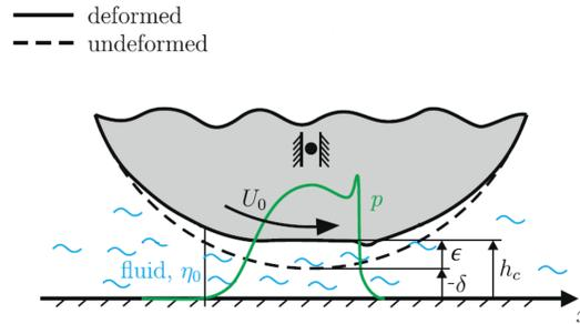
Fig. 1: Contact penetration arrangement [7]
