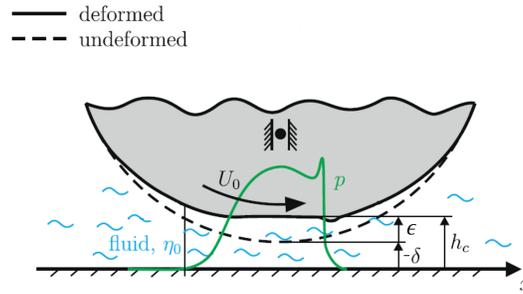
Fig. 1: Contact penetration arrangement [7]
