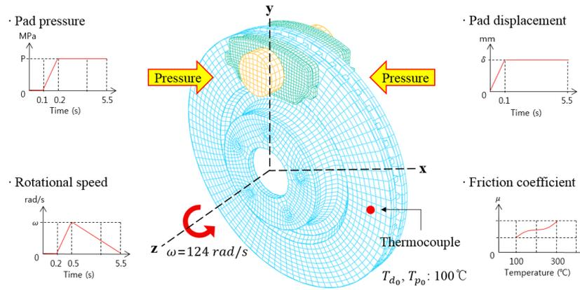
Fig. 2: The finite element analysis model and boundary conditions of the three-dimensional braking system.
