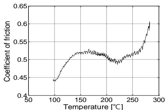
Fig. 1: Temperature-dependent nonlinear friction coefficient.
