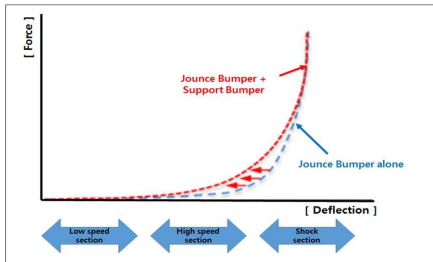
Fig. 1: Load-Deflection characteristic curve of jounce bumper and jounce bumper assembly
