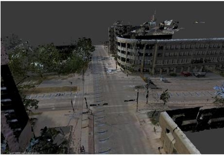
Fig. 1: Mesh generated for Synchrono from LiDAR, camera, and GPS measurements, courtesy of Mandli Communications
