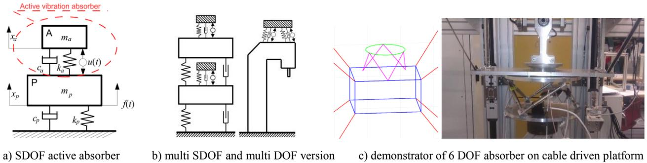
Fig. 1: Active vibration absorber concepts and demonstrator
