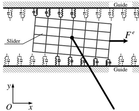
Fig. 1 The frictional translational joint with a flexible slider and clearance
