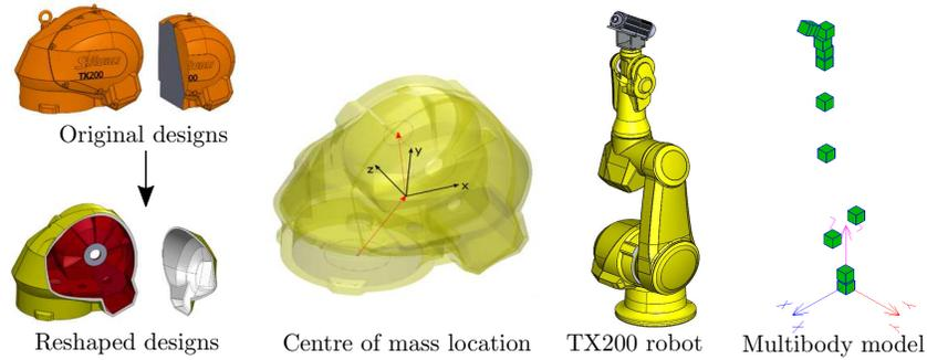
Fig. 1: Modelling steps of the robot dynamic model
