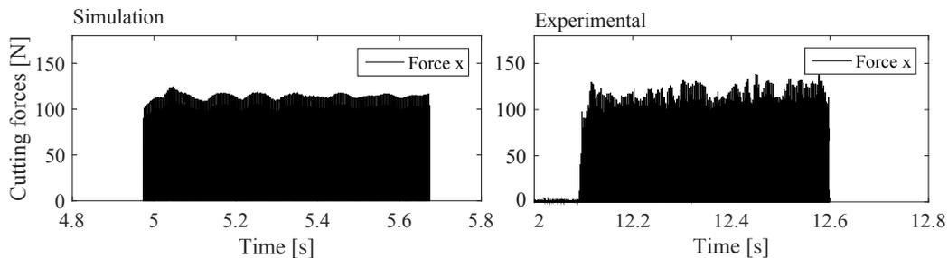
Fig. 2: Comparison of cutting forces (bushings and backlash included)
