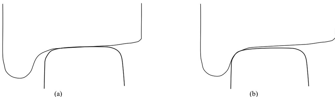
Fig. 1: Wheel-rail contact interaction: (a) non-conformal and (b) conformal scenarios
