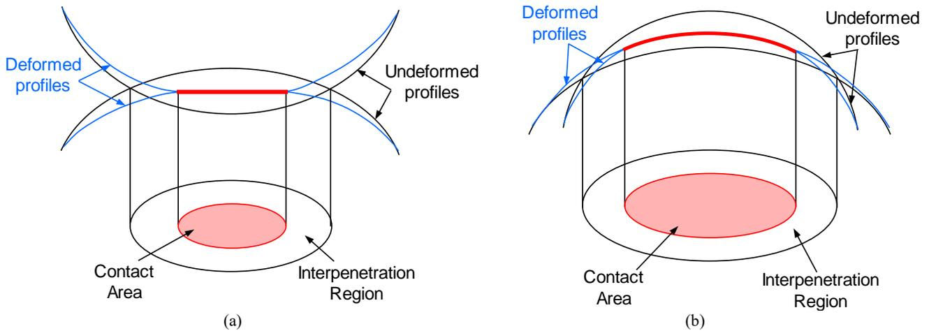
Fig. 2: Schematic representation of the contact region for (a) a non-conformal case (plane contact patch) and (b) conformal case (curved contact patch)
