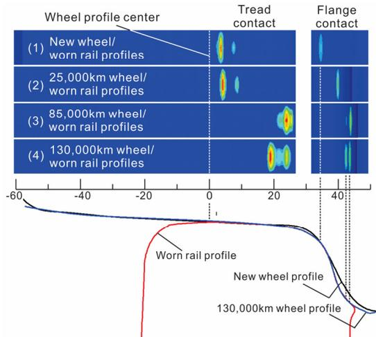
Fig. 1: Contact patches of severely worn wheel and rail
