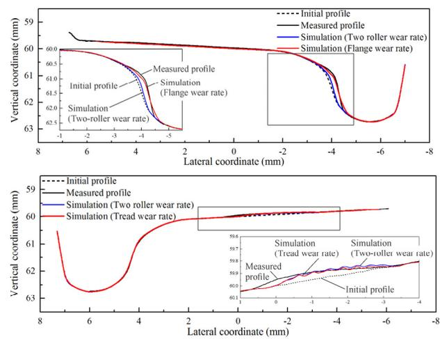
Fig. 2: Wear prediction and comparison with the test data
